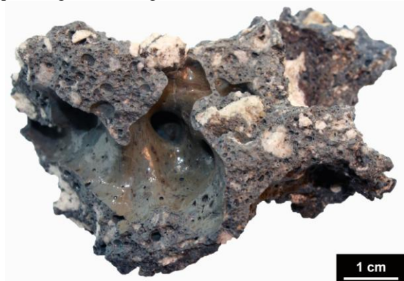
Fig. 2. Photograph of a typical vesicular impact-melt glass fragment from Wabar with partially fused clasts (whitish) of the target material (NHM-Vienna sample L4401).
