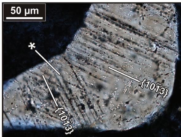
**Fig. 2:** Photomicrograph (in cross-polarized light) of a quartz grain, in a shatter cone from “CS”, containing three decorated PDF sets; one set (\*), with  $\omega'$ {01 1 3}-equivalent orientation, is hardly visible on this photomicrograph, but is evident under the U-stage.
