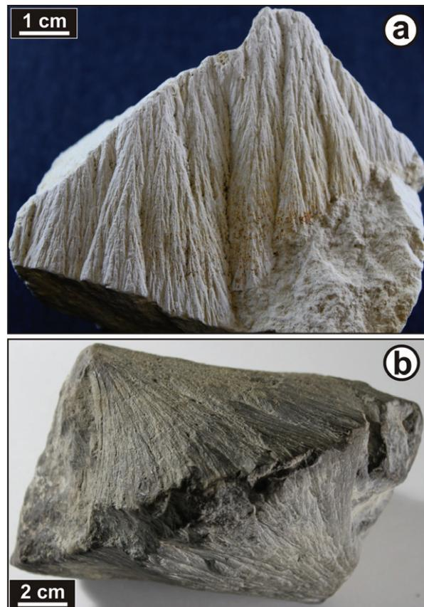
**Fig. 1:** Macrophotographs of shatter cones in limestone. a) Horsetailing shatter cone surfaces (“StS”). b) Two complete cones pointing in opposite directions. Clast from crater-fill impact breccia (“HS”).
