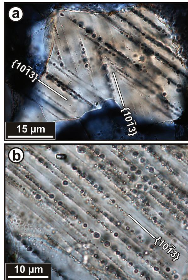
**Fig. 1:** Photomicrographs (in cross-polarized light) of shocked quartz grains in shatter cone sample VN3 from the Keurusselkä impact structure. a) Quartz grain containing two decorated PDF sets with  $\omega\{10\bar{1}3\}$ -equivalent orientations. b) Highly decorated PDF set with  $\omega\{10\bar{1}3\}$ -equivalent orientation.
